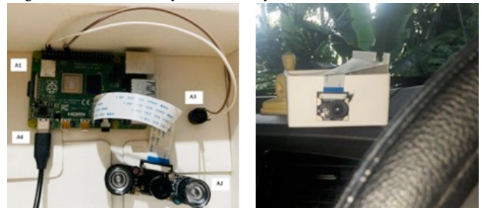
Fig. 8. Drowsiness detection system (a) (A1) Raspberry Pi 4 Model B, (A2) Raspberry Pi Night Vision Camera, (A3) Buzzer, (A4) Power supply
